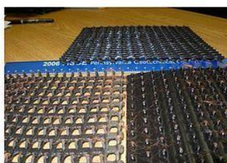
(c) Other geonets (boxshaped channels and protruding columns)
