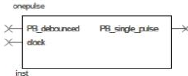
Σχήμα 48 FPGAcore OnePulse: Pushbutton Single Pulse
