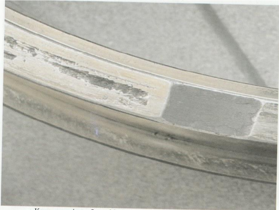
Ring damage due to foreign particles of hard material.
