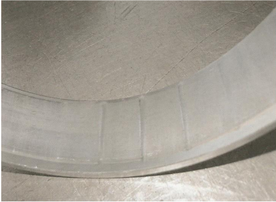
Brinelling in a stand-by machine due to external vibrations.
