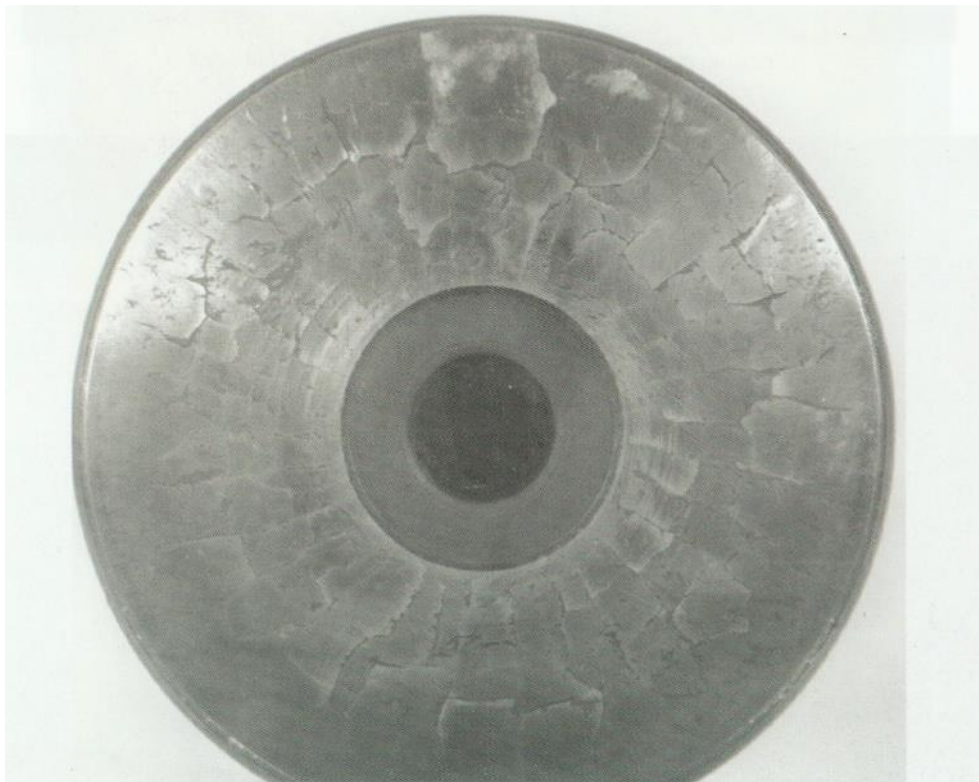
Roller damage by overheating from high load and marginal lubrication.
