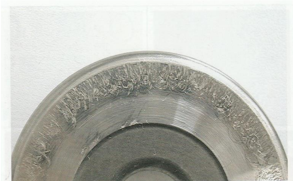
Typical wear on a lateral rolling body surface
