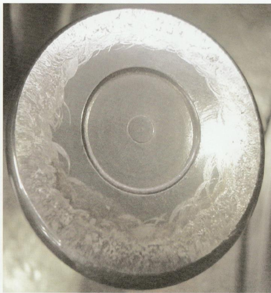
Scrolling phenomenon in lateral surface of the rolling body.
