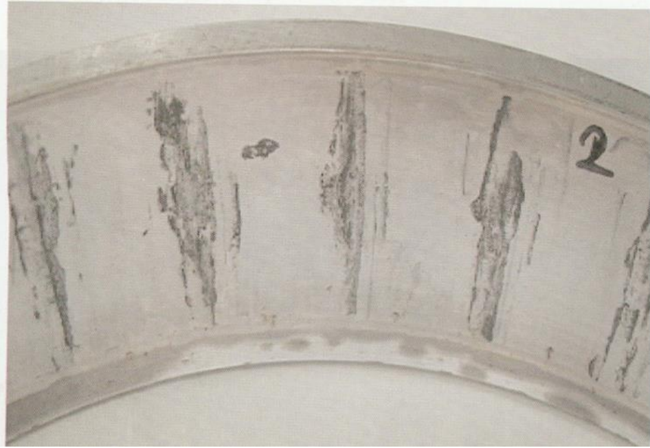
Cage wear due to the existence of water in the lubricant due to poor sealing.
