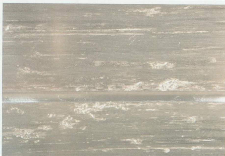
Engravings from foreign particles and small cavities.
