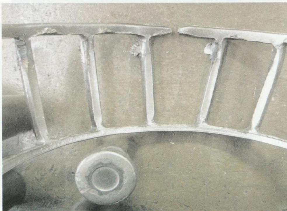
Cage disaster due to obliquities of the rolling body position in motion inverse.
