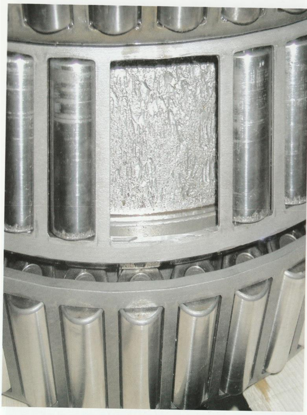
Local cage and rolling bodies damage due to Spalling.
