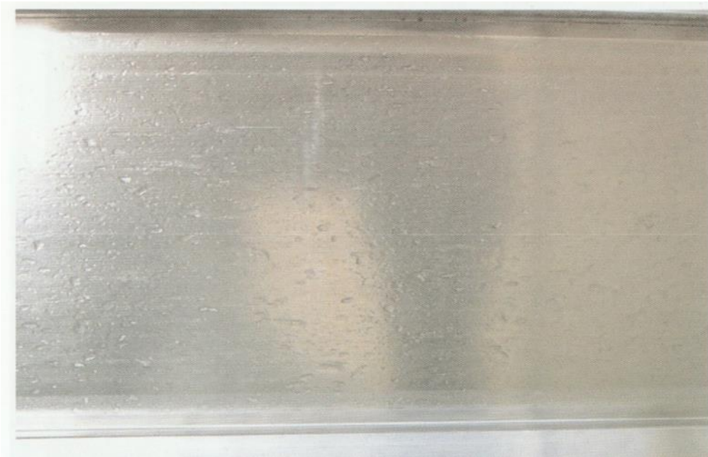
Pits due to foreign particles or by particles from Spalling of the bearing.
