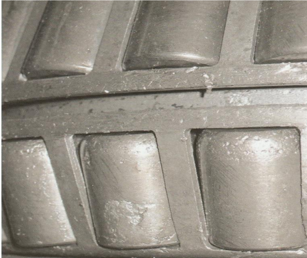
Rolling body and cage damage from Spalling.
