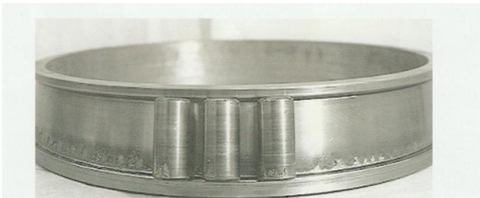
Wear from load unevenness from cone-ring misalignment.
