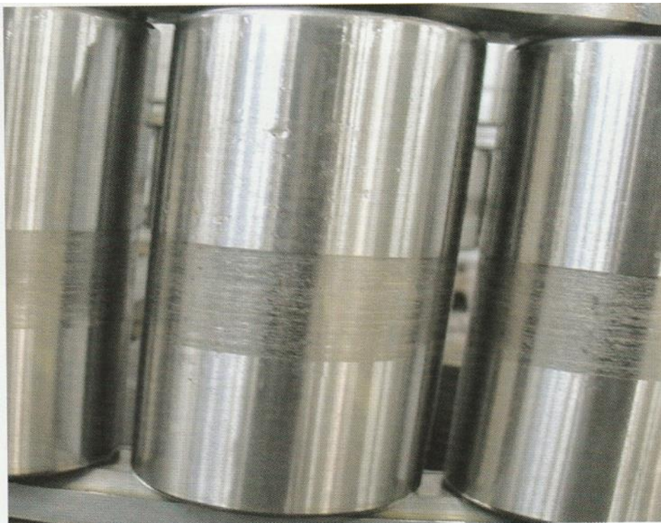
Spall of rolling bodies due to poor lubrication
