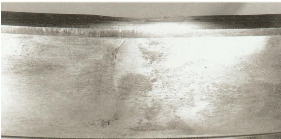
Ring breakage and uneven load due to poor bearing support.
